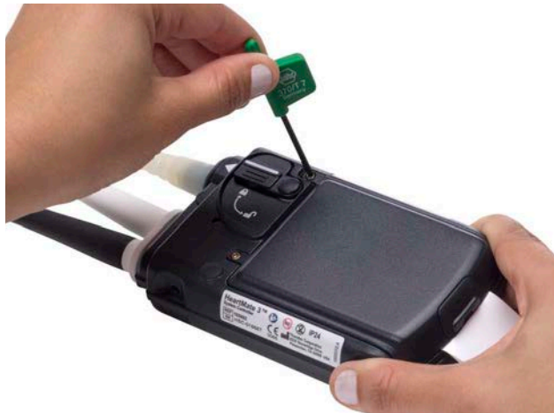
Figure 2.26 Use the Screwdriver to Loosen the Screws
