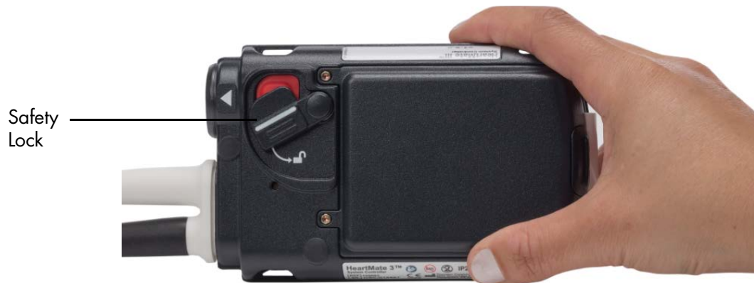
Figure 2.9 Move the Safety Lock to the Unlocked Position
