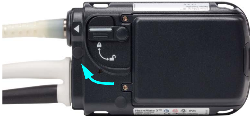
Figure 2.56 Closing the Safety Lock
