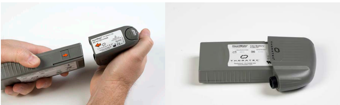
Figure 3.57 Inserting Battery into Battery Clip
