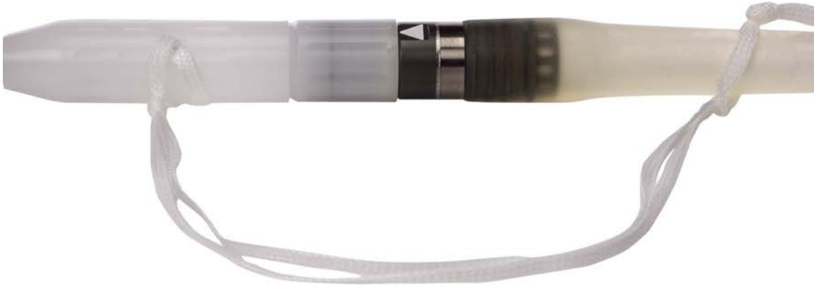
Figure 5.26 Securing the Connection between the Tunneling Adapter and the Pump Cable Inline Connector
