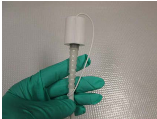
Figure 5.15 Covering the Inline Connector with the Cap
