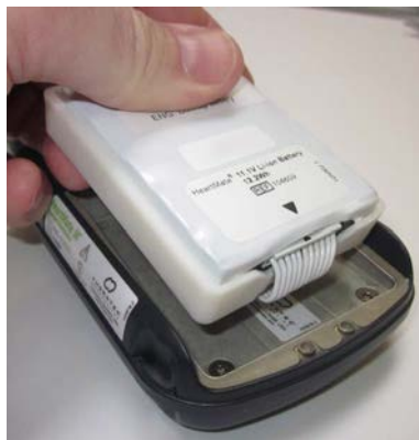
Figure 2.27 Remove Ribbon Cable from Battery Socket
