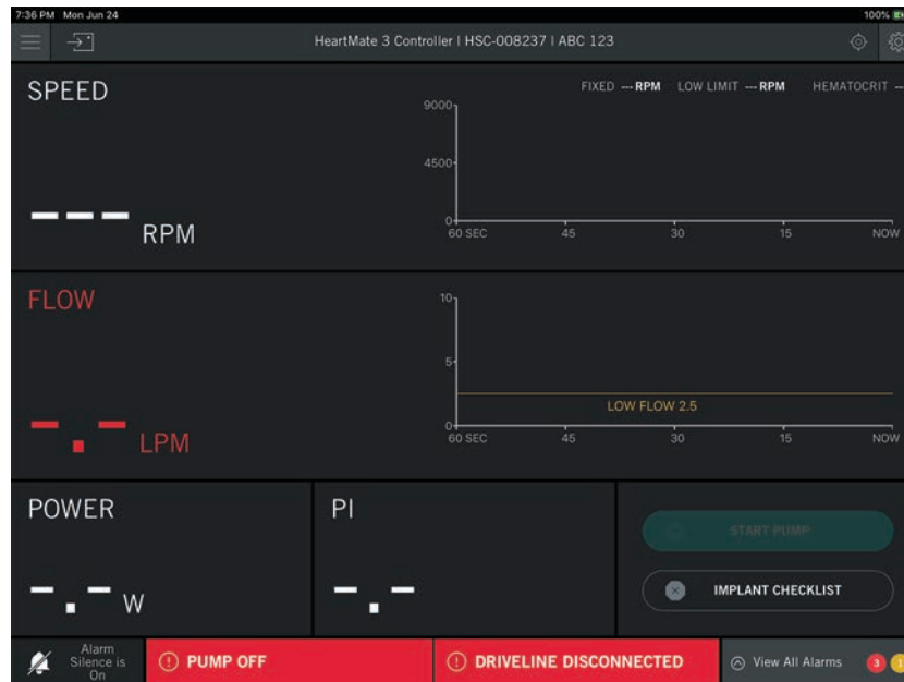
Figure 4.53 Alarms When Driveline is Disconnected
