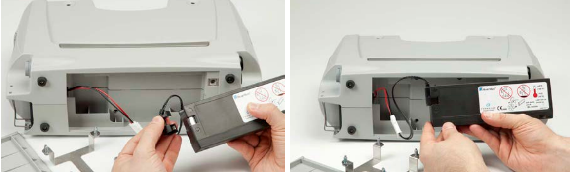
Figure 3.5 Secure the Battery to the Battery Connector
