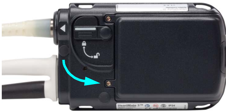
Figure 2.52 Unlock the Safety Lock
