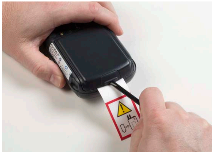
Figure 5.49 Use the Lever to Lift up the Cover
