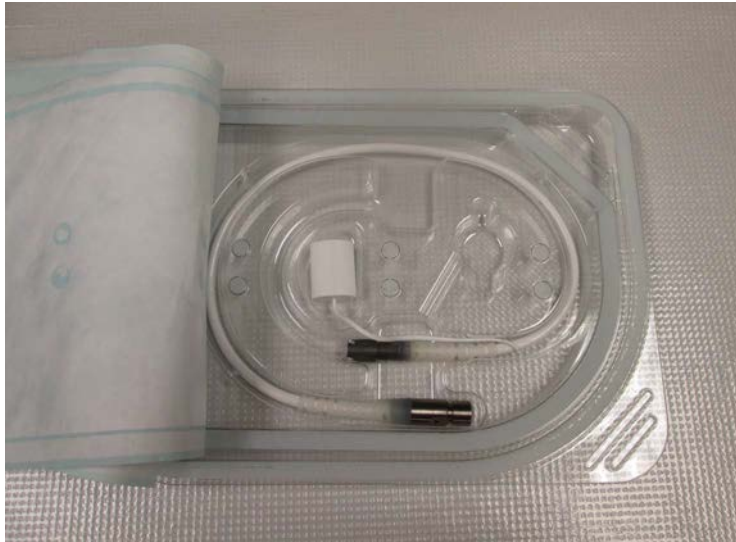
Figure 5.14 Outer and Inner Plastic Trays with Lids Peeled Back from Modular Cable
