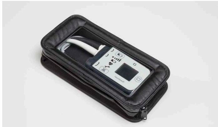
Figure 6.55 Protection Bag with Backup Controller and Cables Stored Inside
