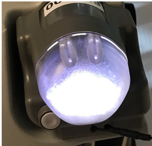
Figure 4.8 HeartMate Touch Wireless Adapter Light Flashes White
