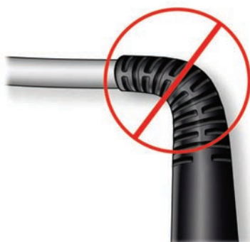
Figure 6.59 Do Not Bend System Controller Power Cables
