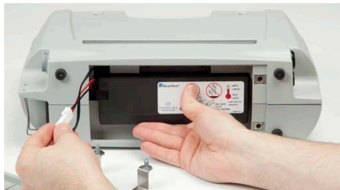
Figure 3.6 Place the Battery in the Battery Compartment
