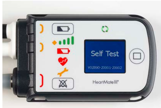
Figure 2.17 User Interface During System Controller Self Test
