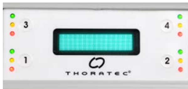
Figure 3.71 Display Panel During Battery Charger Self Test
