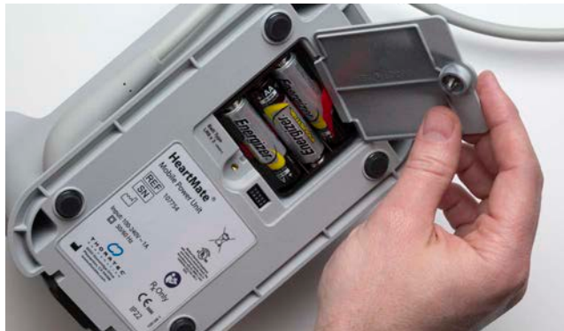
Figure 3.42 Remove the Battery Compartment Cover
