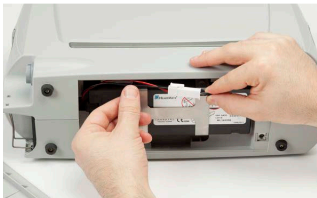
Figure 3.30 Gently Pull the Wires and Connectors Away
