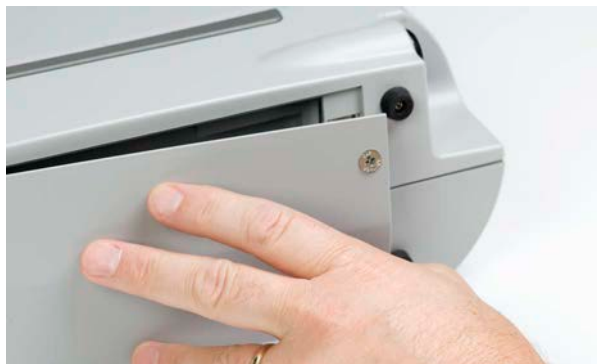
Figure 3.35 Remove the Battery Compartment Cover
