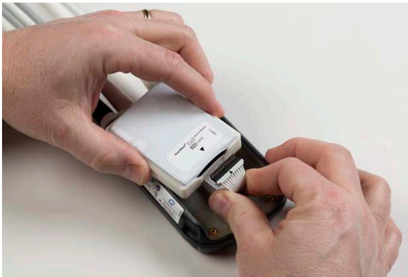
Figure 5.51 Align the Arrow on the Cable with the Arrow on the Battery
