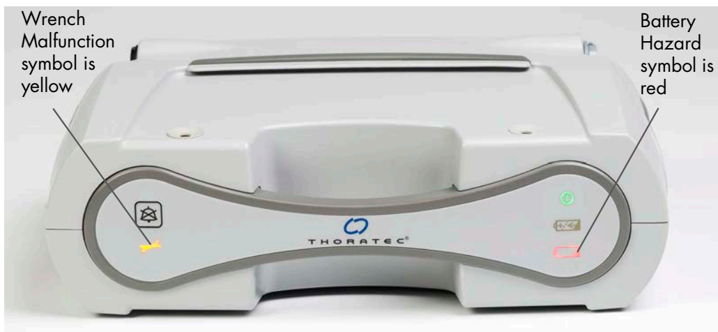
Figure 3.27 Yellow Wrench and Red Battery Hazard Symbol Indicate that the Power Module Backup Battery is Not Working — Switch to Another Power Source Immediately
