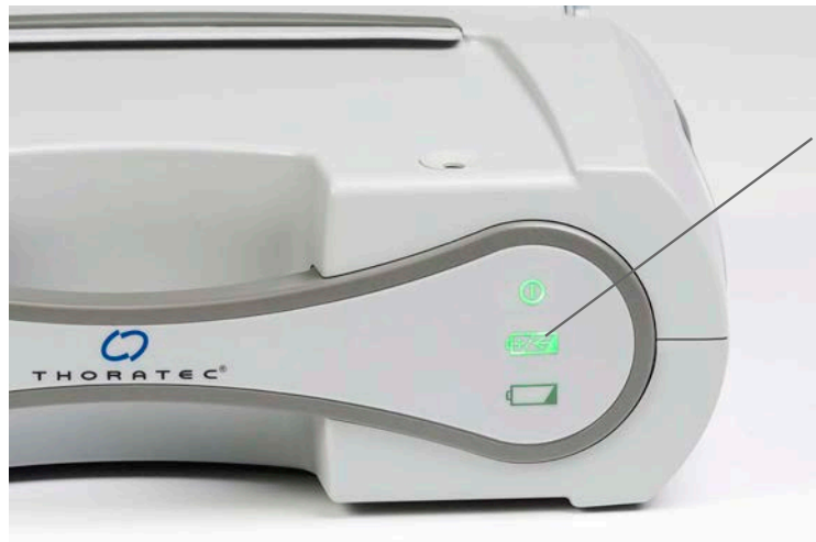
Figure 3.24 Green Charge Symbol Indicates that the Power Module Backup Battery is Charged
